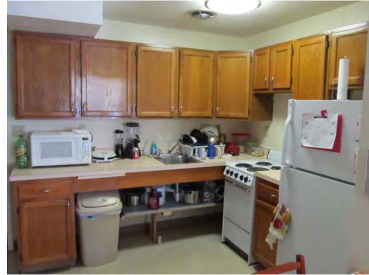
Handicap accessible unit kitchens include knee clearance space under sink and at work surface but countertop exceeds height limit above floor
